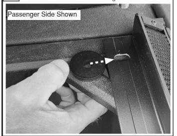
Align the black washer's hole to the side rails oblong hole. Move the front header in place and align the screw in the header with the hole in the rail and washer. Drop the header down so the screw extends through the holes.
